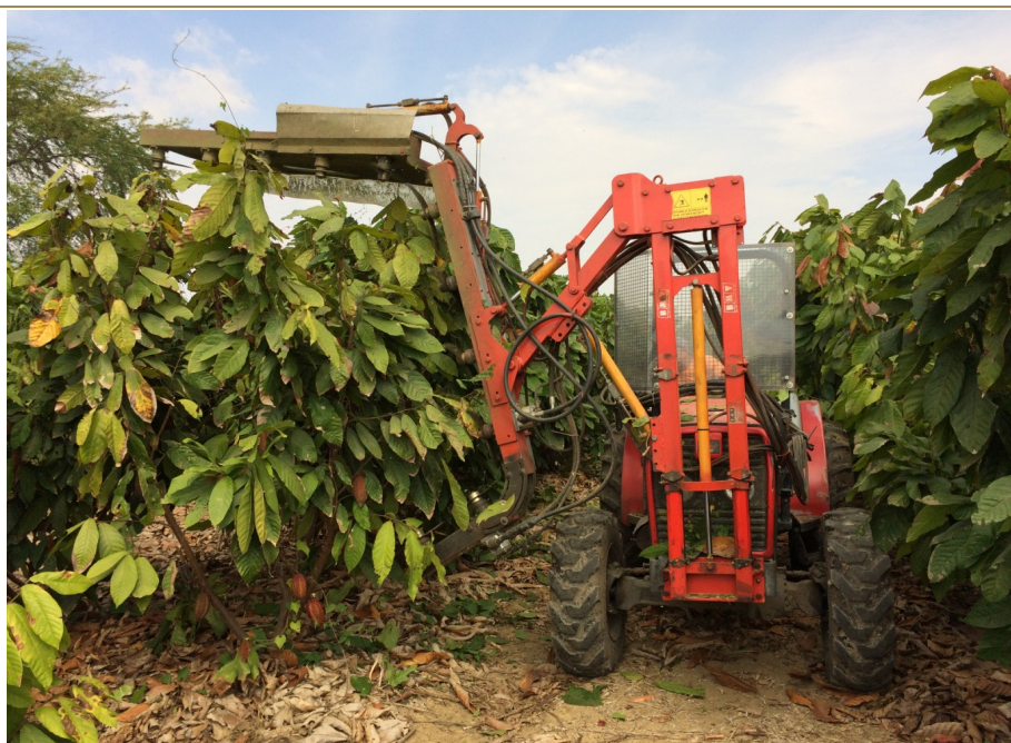
Source: A mini-tractor and pruning arm managing CCN-51 tree height and morphology in Ecuador. Photograph supplied by Roberto Mollison.
